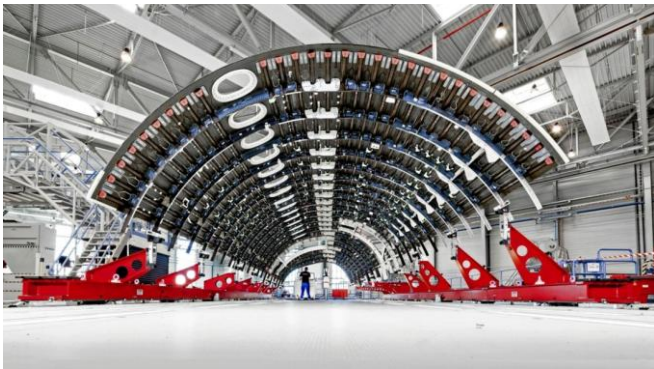
Figure 1: Fuselage shell of the Airbus A350 made of carbon fiber reinforced plastic [2]
