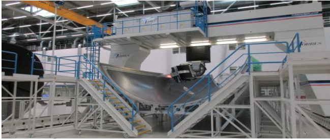
Figure 3: AFP Process for Panel production (picture PAG)
