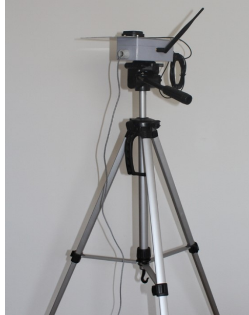
Figure 2. DGNSS Base Station with GNSS antenna and radio transmitting antenna
