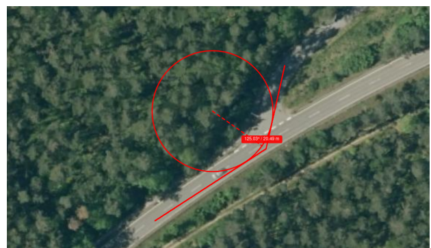
Figure 1. Example intersection with speed limit 80 \frac{km}{h} , 20 m radius and flat branching street [8]
