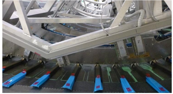
Figure 5: Positioning the stringers on the aircraft panel (picture PAG)
