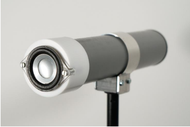
Fig. 3. Special loudspeaker used for Localization testing
